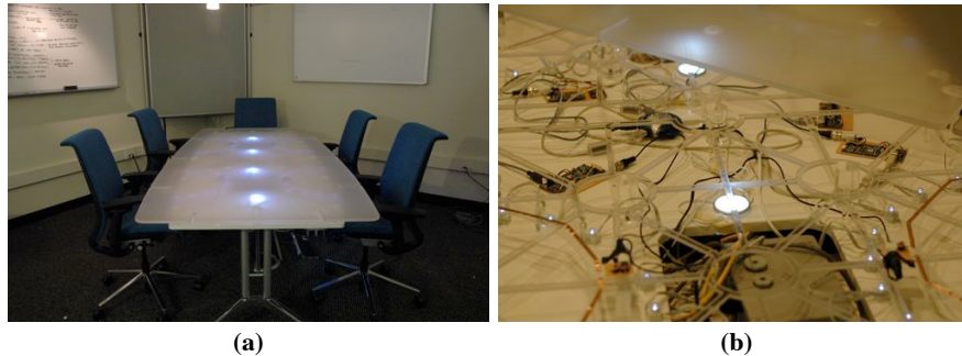
Fig. 3. The inSpace Table, displayed (a) as situated in the meeting room environment, and (b) with the translucent top layer removed to expose the internal structure and configuration.
